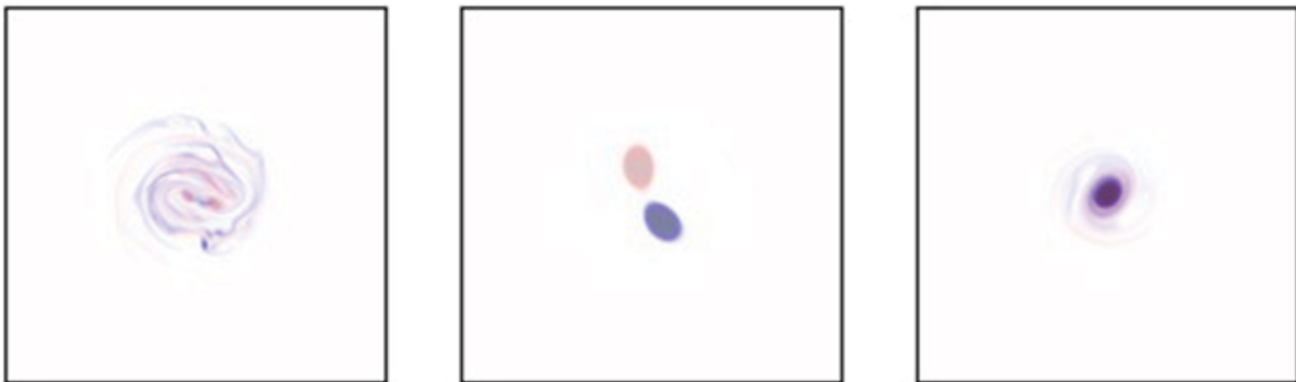
Figure 1: Top view over the upper and middle layers of a three-layer system at t = 349 for a basin (left), a flat bottom (middle) and a seamount (right). Vortices are initially distant by 3.5 times their radius. Their radius is 3 times the deformation length in each layer. The Gaussian seamount/basin has a characteristic radius 3 times the one of the vortices.
